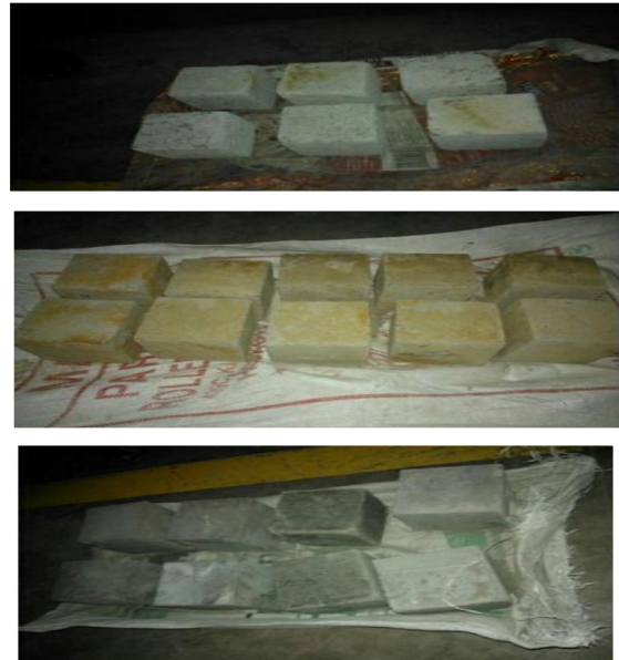
Fig 4: Cubes after 1) Acid attack test, 2) Sulphate attack test, 3) Chloride attack test
