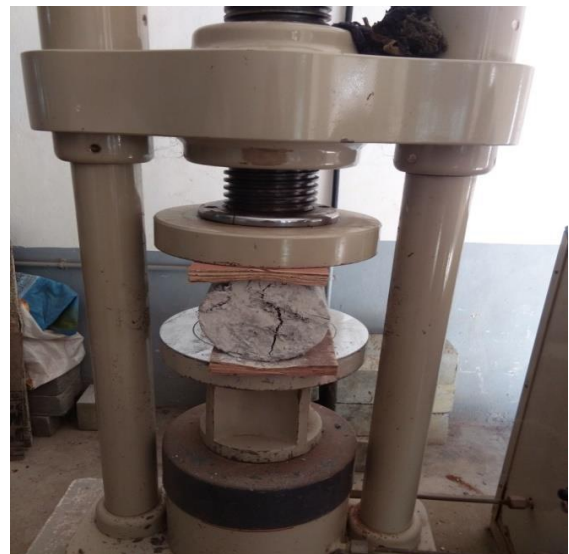
Fig 3: Split tensile strength testing with sample
