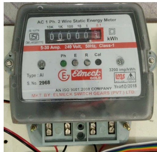
Fig 6.Single Phase Energy Meter
