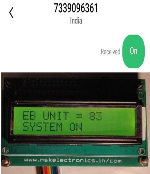
Fig 12.ON Process of Energy Meter
