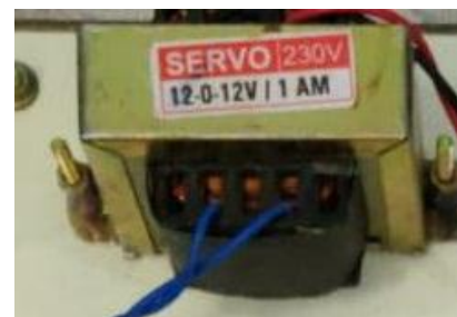
Fig 4. Current Transformer (230/12 v)
