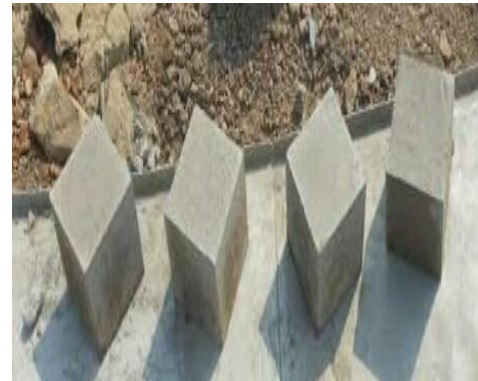
Fig. 4. Demoulding of Concrete
