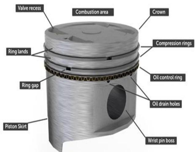
Fig.1 Piston Head Assembly
