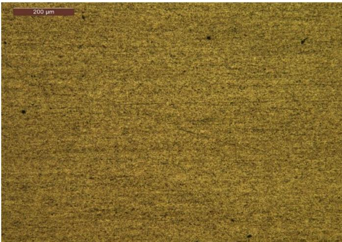
**Fig.33** Microstructure of Uncoated Specimen for Mag.500X
