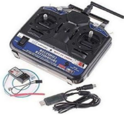
Fig 8. RC Transmitter & Receiver
