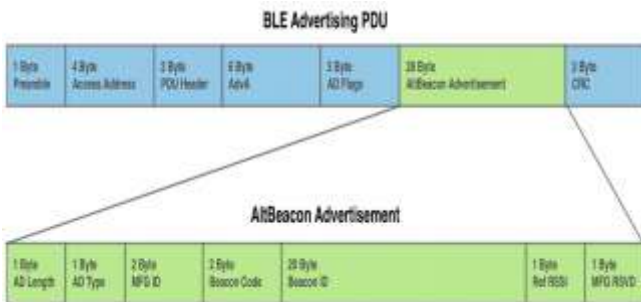
Fig. 2. AltBeacon data structure [3]
