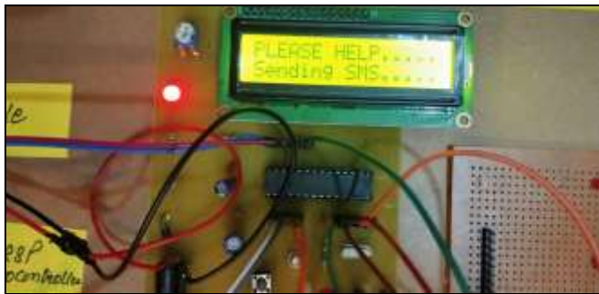
Fig -7: Danger Zone: "Please help" message displayed on the LCD screen same will be messaged to the predefined number
