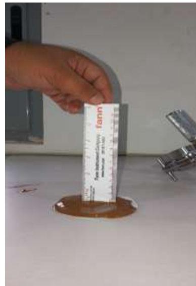
Fig -4: Mud cake thickness scale (Fann)
