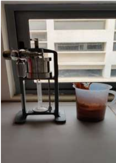
Fig -1: API LPLT filter press (Fann)
