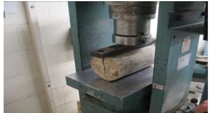
Fig-5: Split tensile strength
