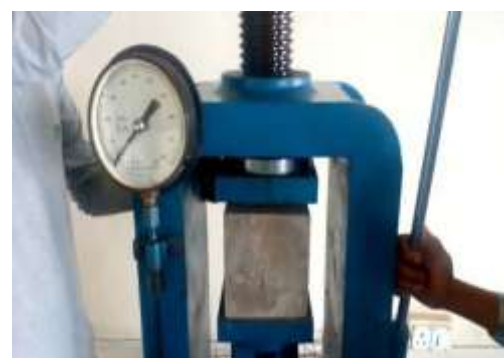
Fig-4: Compression strength
