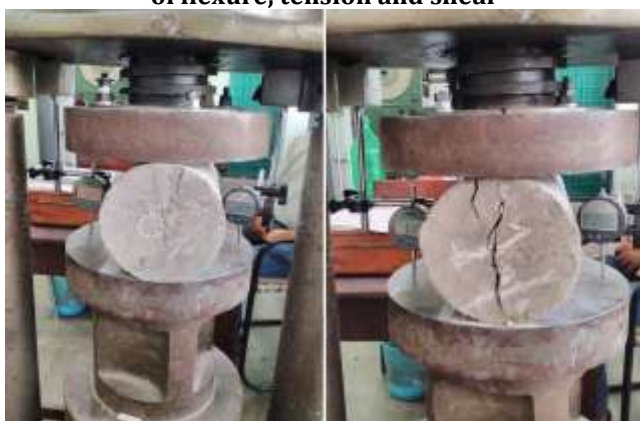
Fig. 3 Arrangement for testing Cylinders for splitting Fig.
