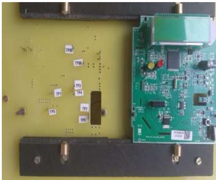
Fig: Smart Energy Meter Test Jig with Meter board and Testing Pins.
