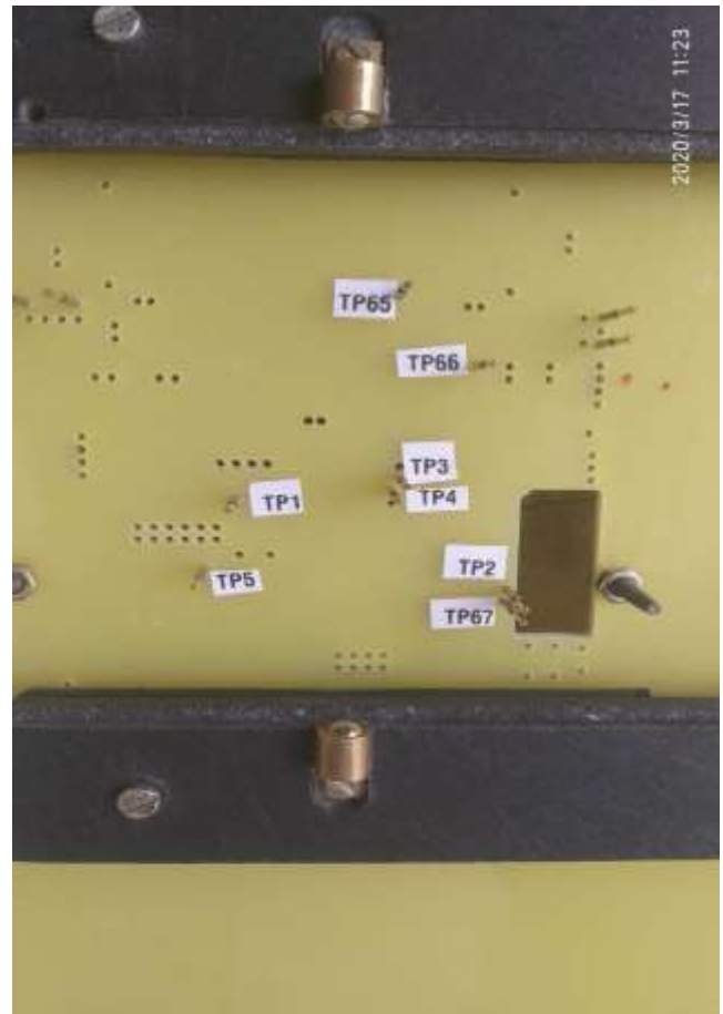
Fig: Main Board with Testing Pins
