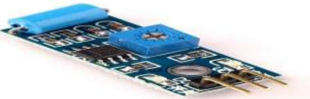
Fig-6: Vibration sensor for accident detection
