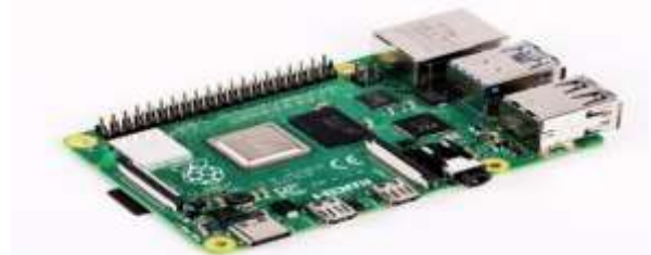
Fig-4: Raspberry Pi 4 for drowsiness detection
