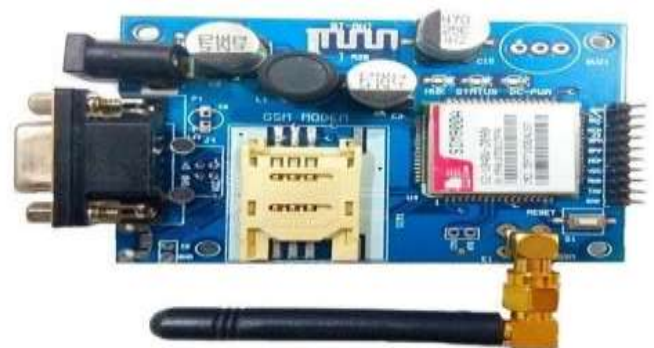
Fig-8: GPRS module for sending alert to family members
