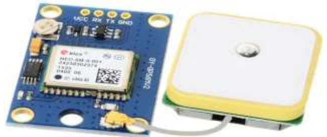
Fig-7: GPS sensor for tracking vehicle
