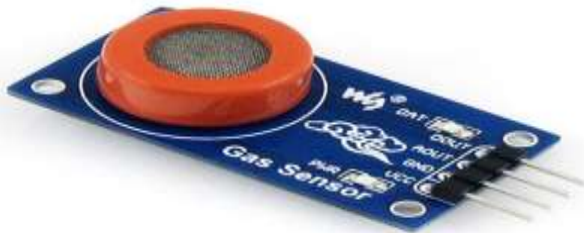
Fig-5: MQ-3 sensor for alcohol detection
