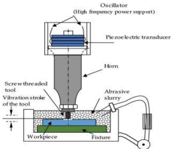
**Fig -1:** Ultrasonic machining process
