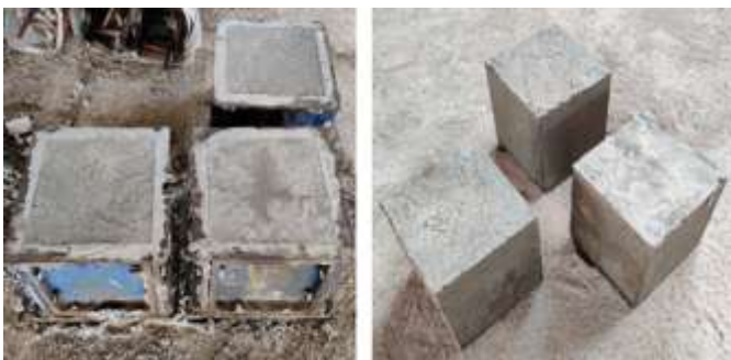
Fig -11: Concrete cubes dried and ready for curing
