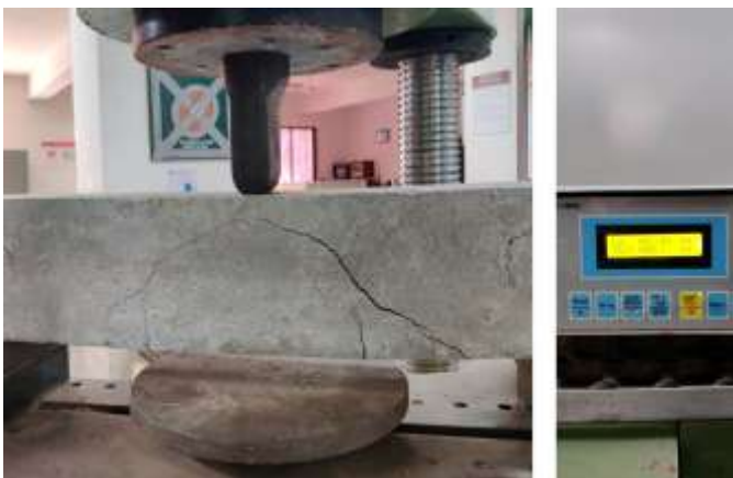
Fig -22: SB SRCC beam breaking point with reading
