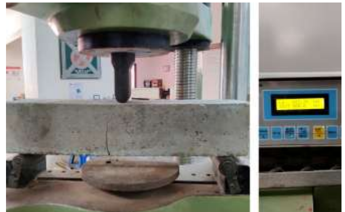
Fig-20 : D1 BRCC beam breaking point with reading
