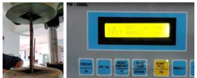
Fig -16: Dagdi bamboo specimen under UTM and readings
