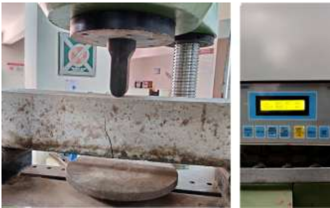
Fig -21: M2 BRCC beam breaking point with reading
