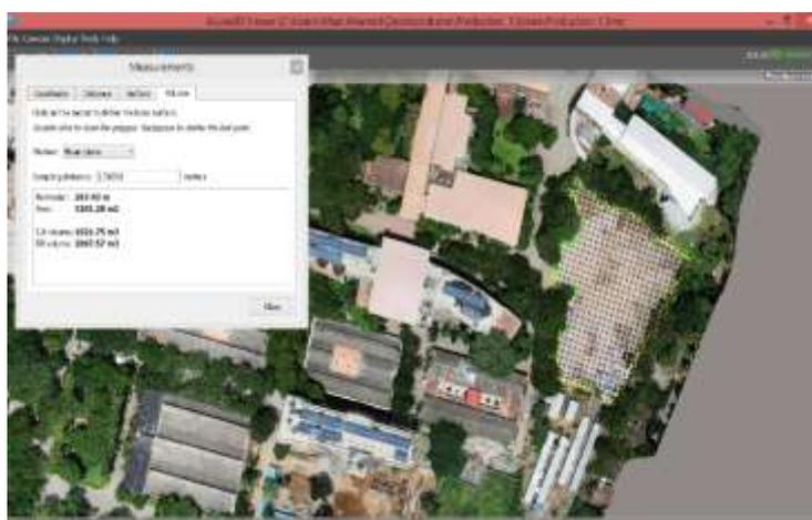
Figure 18. Cut and Fill volume of Empty land for construction
