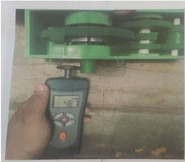
Fig 9: Tachometer reading showing reduction of 4:1
