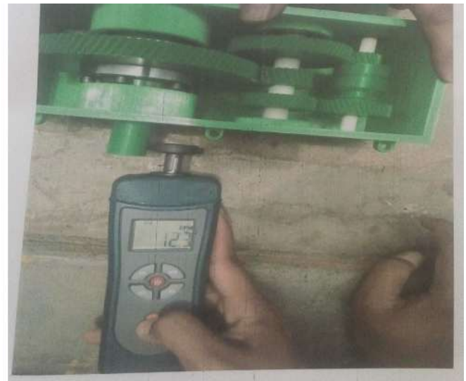
Fig 7: Tachometer reading showing reduction of 16:1
