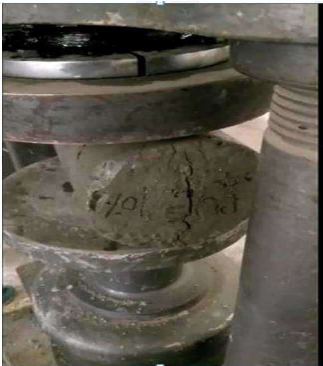
Fig(g): Testing of cylinder specimen
