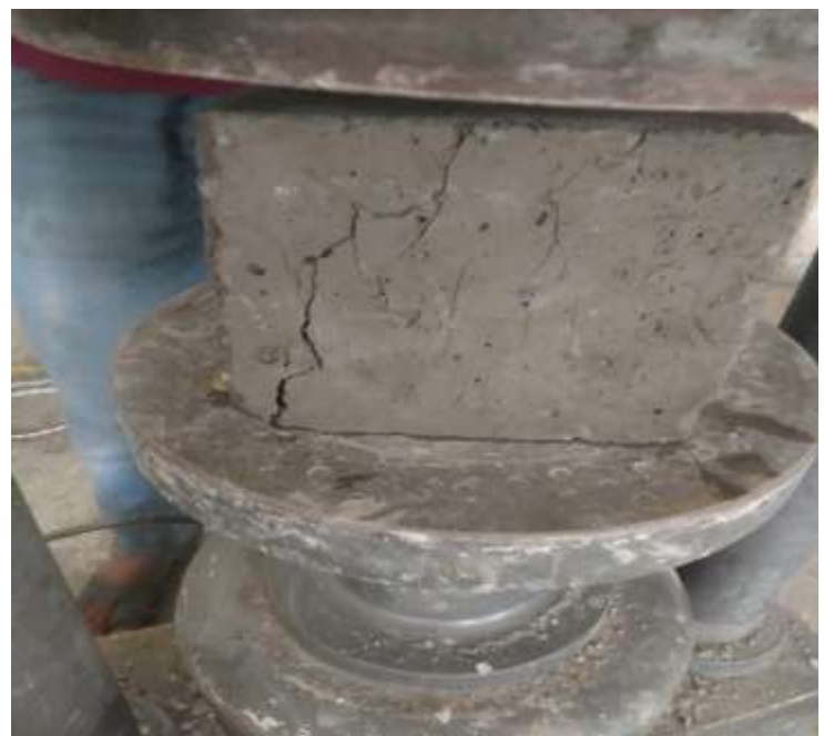
Fig (f): Compression test of cubes
