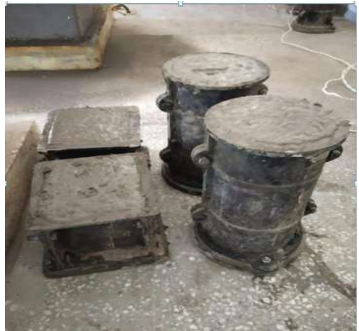
Fig (e): Casting of cylinder moulds
