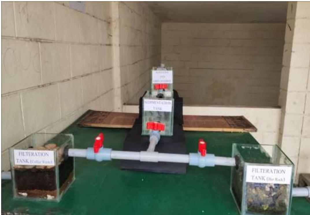
Fig 6 – Working model of wastewater treatment system
