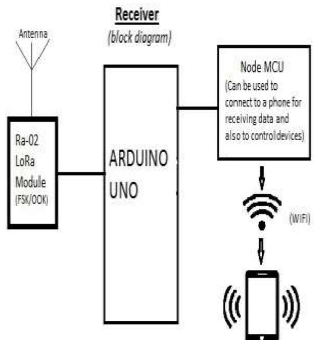
**Fig -3:** Receiver side Block diagram
