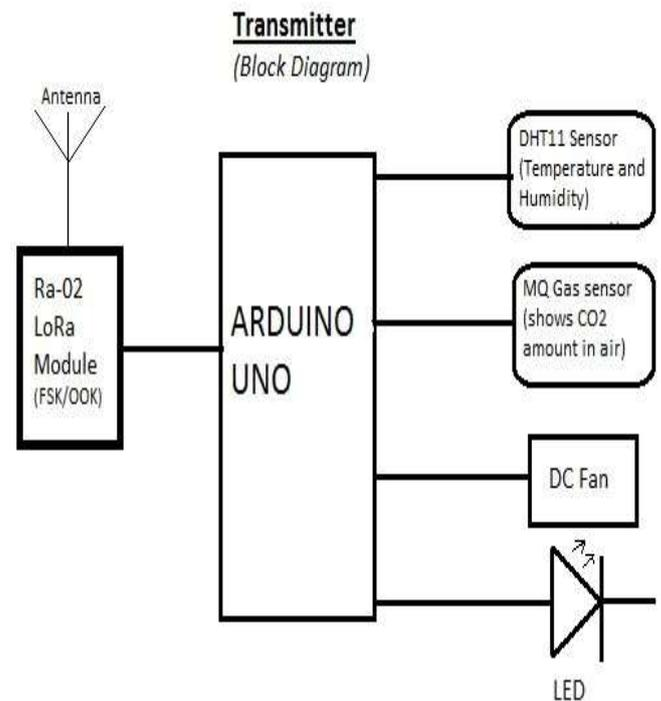
**Fig -2:** Transmitter side block diagram
