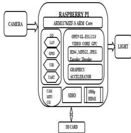
**Fig 3. ARCHITECTURE DIAGRAM**
