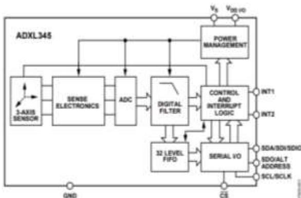
Fig 2: Functional Block Diagram [8]
