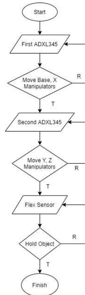
Fig-3: Block Diagram of Robotic Arm
