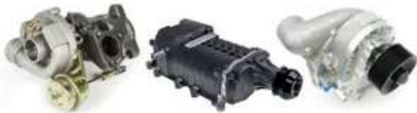
Fig 6: Turbo, Roots type and Centrifugal Supercharger
