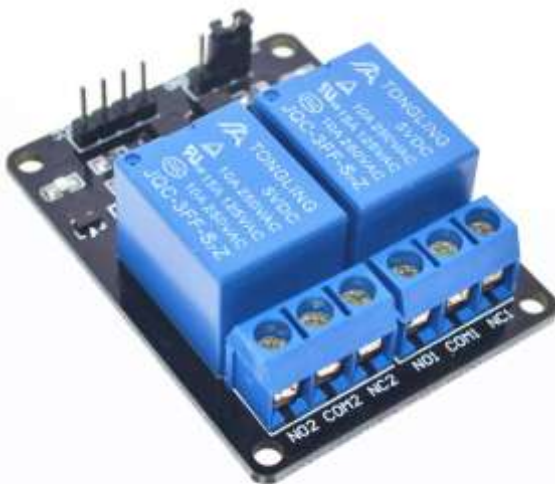
Fig 6- JQC-3FF-S-Z 2-Channel Relay Module
