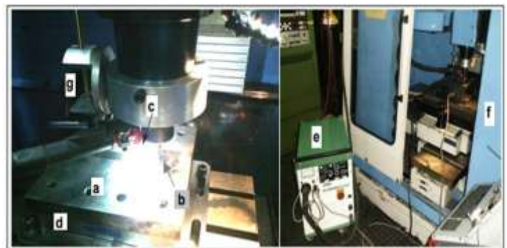
Fig. 3: Experimental equipment of PAM. (a) Inconel 718 or Haynes 25, (b) milling tool, (c) plasma torch, (d) Kistler 9255B force measuring device, (e) plasma generator, (f) 3 axes vertical machining center, (g) torch positioning system (2 axes)
