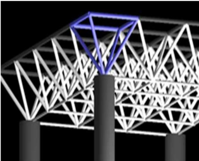
Fig - 1: (a) Space Frame Truss
