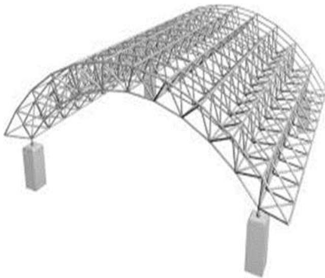
(b) Barrel Vault Space Structure
