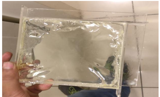
Fig -1. Poured mixture of hardener and resin
