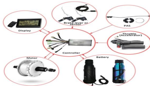
Fig -8: Functioning of the controller
