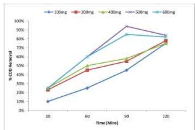
Chart -2: Effect of H<sub>2</sub>O<sub>2</sub> on COD Removal (pH=3, Fe<sup>2+</sup>=400mg)
