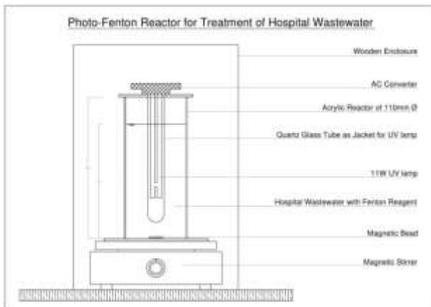
Fig - 2: Photo-Fenton Reactor
