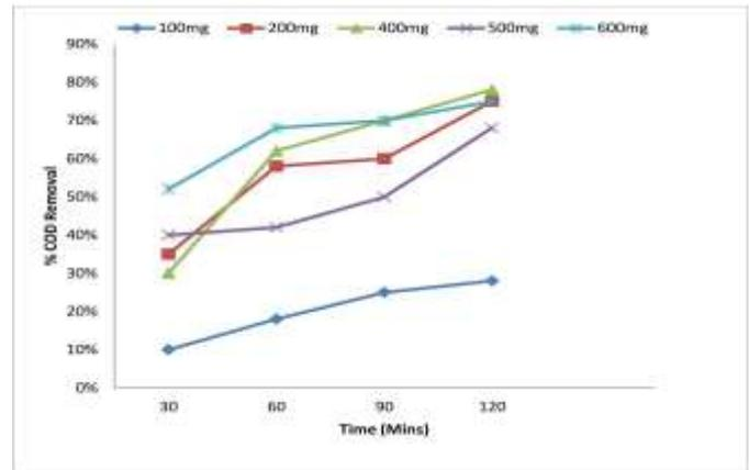
Chart -1: effect of Fe<sup>2+</sup> on COD Removal (pH=3, H<sub>2</sub>O<sub>2</sub>=400mg/l)
