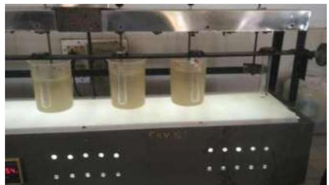
Fig – 1: Fenton process using jar test apparatus
