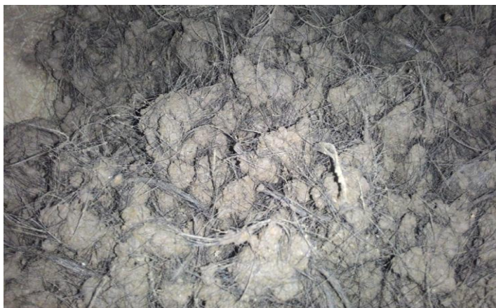
Fig -2: Soil Mixed with Human Hairs
