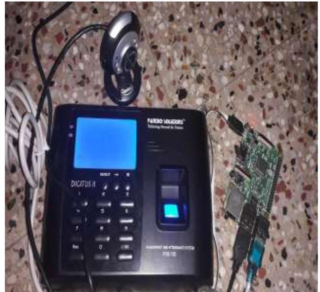
Fig 3: Hardware prototype of fingerprint and face recognition
