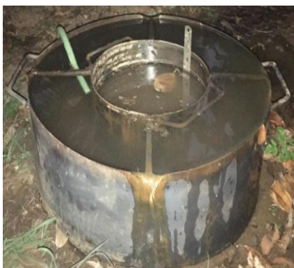
Fig -2: Test conducted on Double ring Infiltrometer
