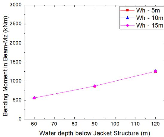
**Chart - 10:** Maximum major axis bending moment in beams of jacket structure
