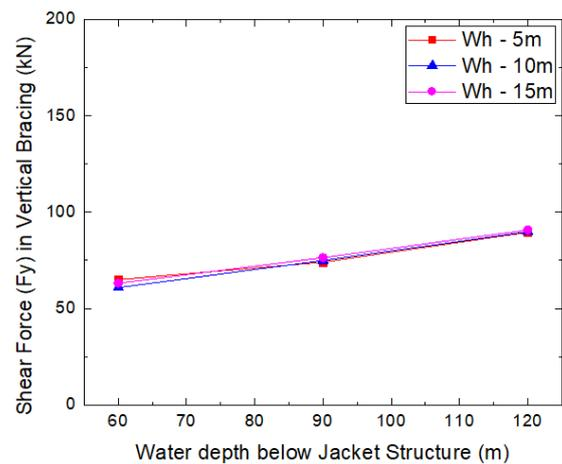
**Chart - 17:** Maximum shear force in vertical bracings of jacket structure
