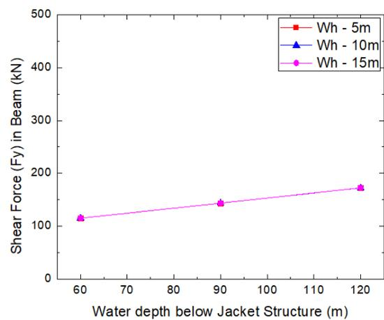
**Chart - 12:** Maximum vertical shear force in beams of jacket structure
