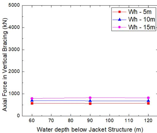
**Chart - 15:** Maximum axial force in vertical bracings of jacket structure
