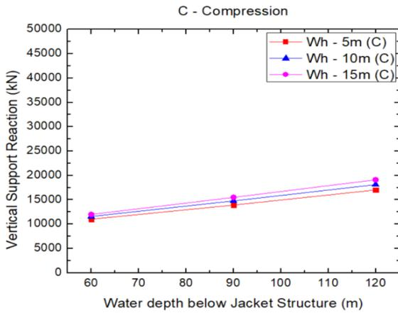
Chart - 3: Maximum vertical support reaction for Jacket structure
