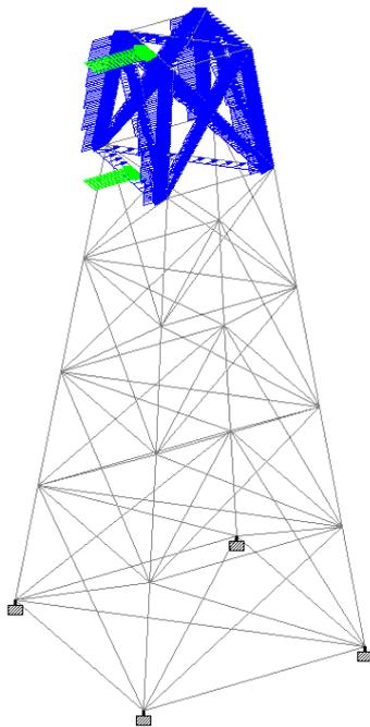
Figure - 3: Application of wind load on Jacket structure and conductors pipes
