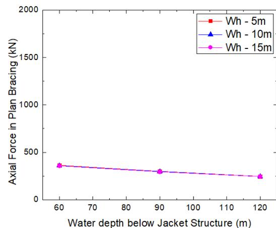
**Chart - 16:** Maximum axial force in plan bracings of jacket structure
