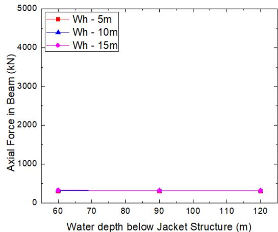
Chart - 8: Maximum axial force in beams of jacket structure
