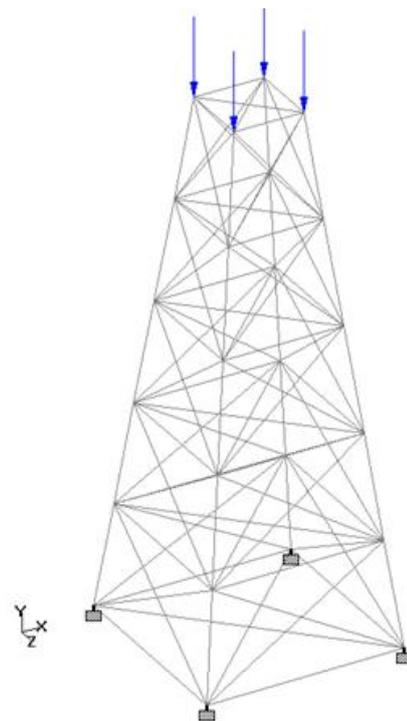
**Figure - 1:** 3-Dimensional STAAD model of Jacket structure with deck load
