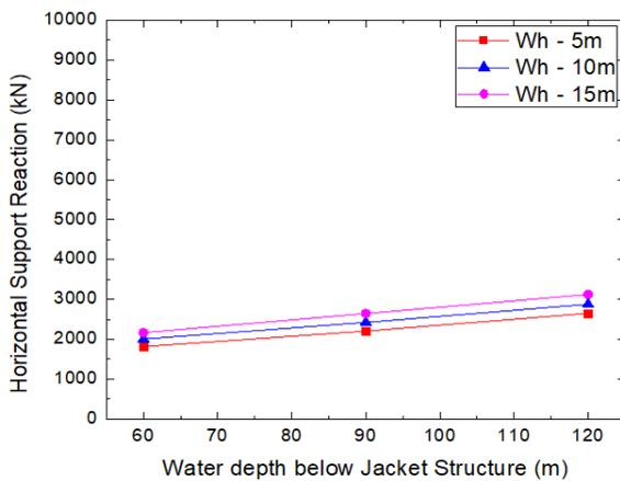
Chart - 5: Maximum horizontal support reaction for jacket structure
