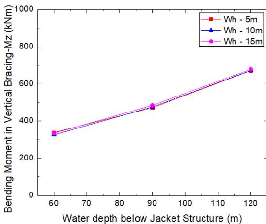
**Chart - 19:** Maximum bending moment in vertical bracings of jacket structure
