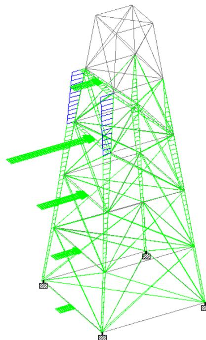
**Figure - 2:** Application of wave & current load on Jacket structure and conductors pipes
