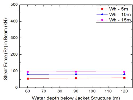
**Chart - 13:** Maximum horizontal shear force in beams of jacket structure
