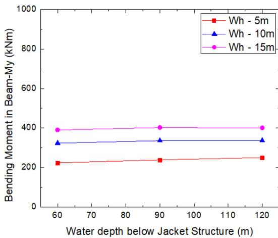
**Chart - 14:** Maximum minor axis bending moment in beams of jacket structure
