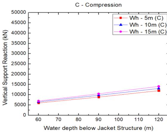
Chart - 4: Minimum vertical support reaction for standalone jacket structure without deck load
