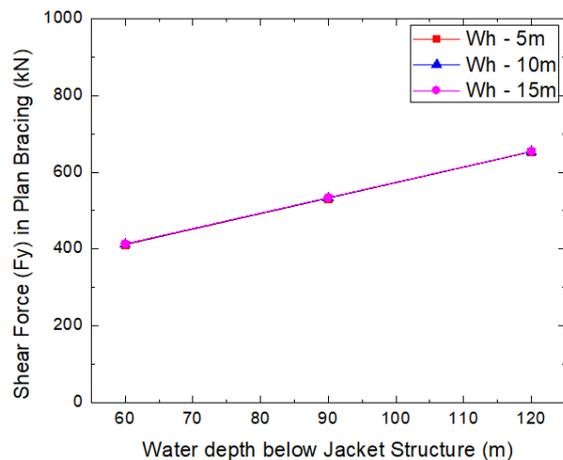
**Chart - 18:** Maximum shear force in plan bracings of jacket structure
