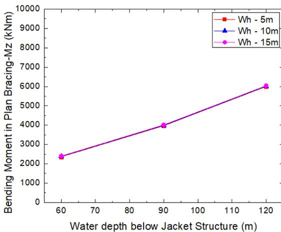
**Chart - 20:** Maximum bending moment in plan bracings of jacket structure
