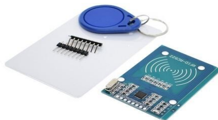
Fig2.6: RFID Reader and RFID Tag
