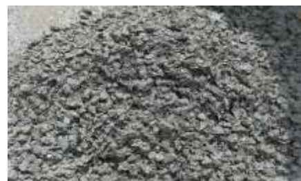
Fig-1 Crushed Bottle Caps added to Concrete
