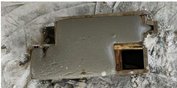
Fig -11: Mold after AC has fully risen
