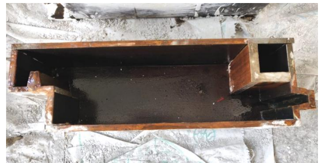
Fig -8: Assembled mold and oiled for pouring of AC mix
