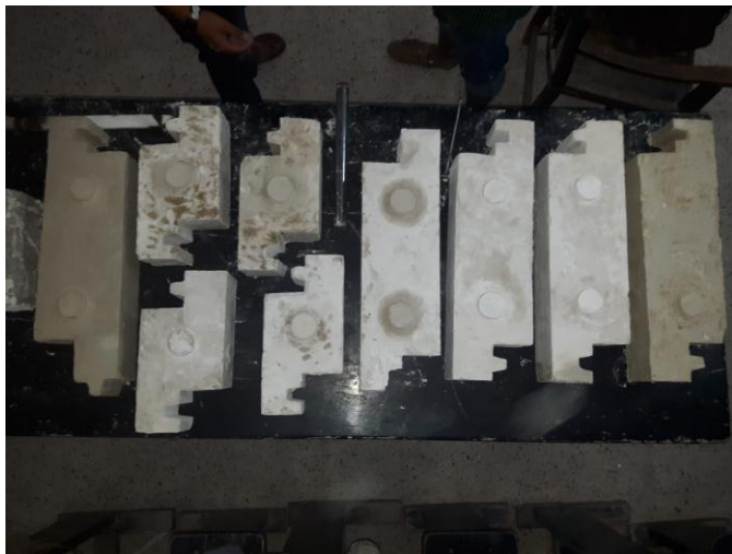
Fig -6: Trial blocks casted for checking suitability of SIB
