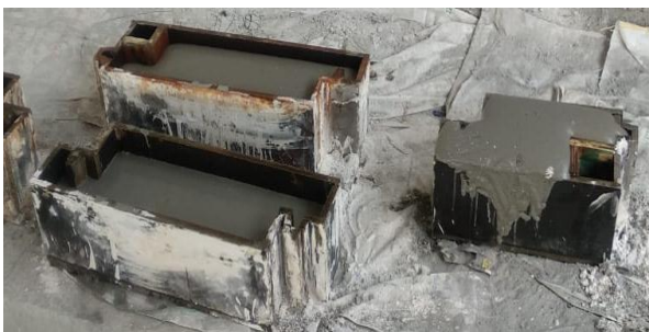
Fig -10: Molds filled up to 2/3 rd height and left for rising
