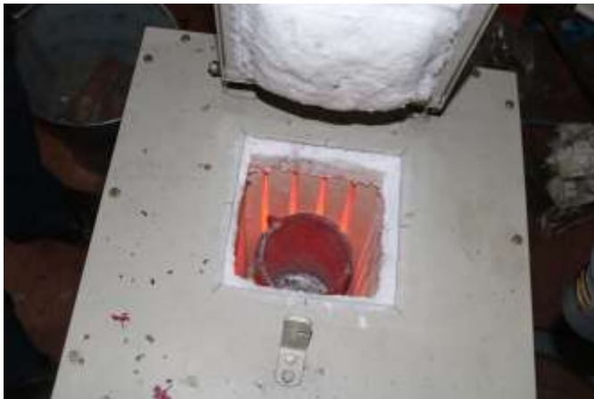
Fig - 1 Induction Furnace
