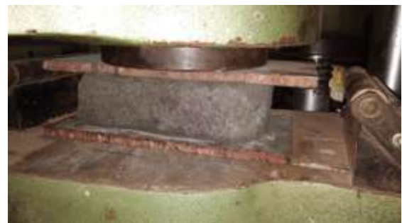
Fig. 2: Compressive Strength test on RHA-Brick block
