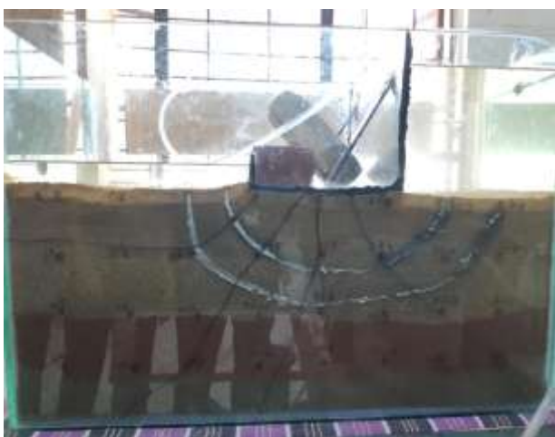
Fig 8.1: Without cut-off wall ( \theta = 0^\circ )
