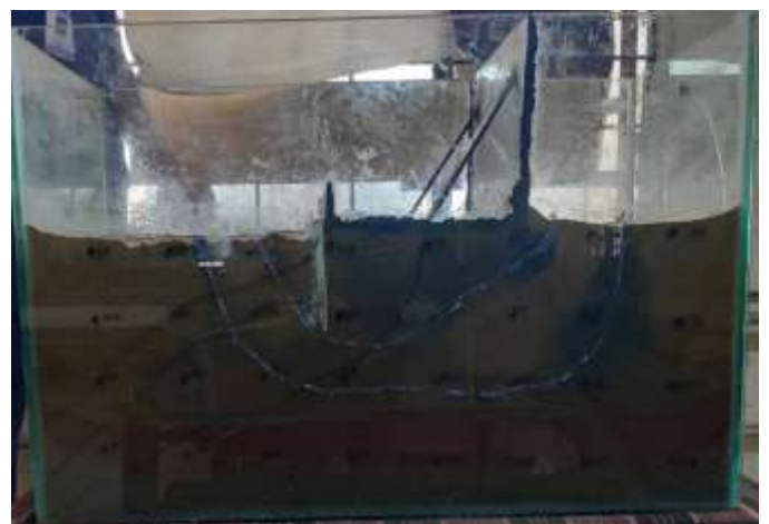
Fig 8.4: Cut-off at downstream side \theta = 90^\circ
