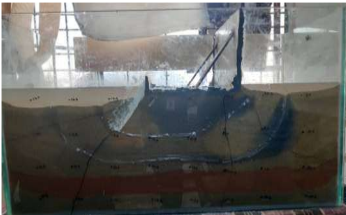
Fig 8.5: Cut-off at downstream side \theta = 120^\circ
