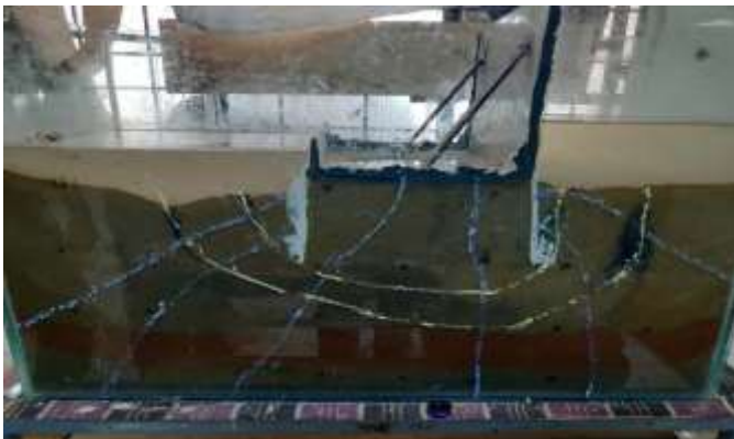
Fig 8.6: Cut-off at both U/S and D/S \theta = 90^\circ
