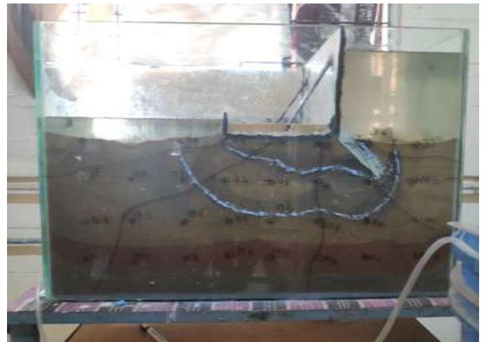
Fig 8.2: Cut-off at upstream side \theta = 45^\circ
