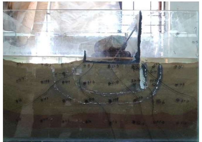
Fig 8.3 Cut-off at upstream side \theta = 90^\circ
