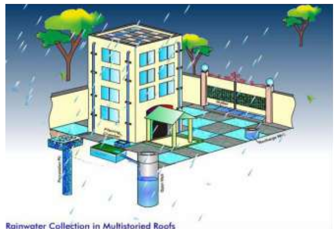
Fig. 2: Rainwater Harvesting System
