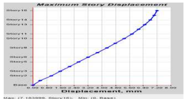
Fig.14 Max. displacement of CSB model 3
