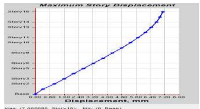
Fig.12 Max. displacement of CSB model 2
