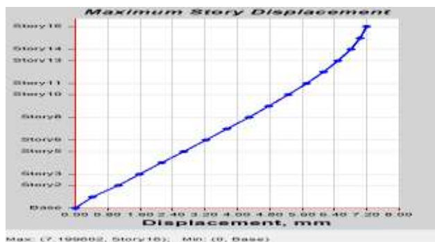
Fig.16 Max. displacement of CSB model 4
