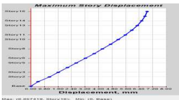
Fig.10 Max. displacement of CSB model
