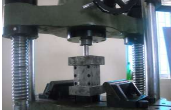
Figure 1.9: Compacting in UTM
