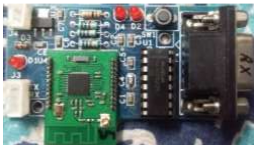
Fig 3. XBee with RSSI module at receiver side
