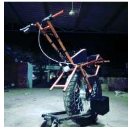
Fig -16: Prototype of self-balancing Electric Uni- Wheeler
