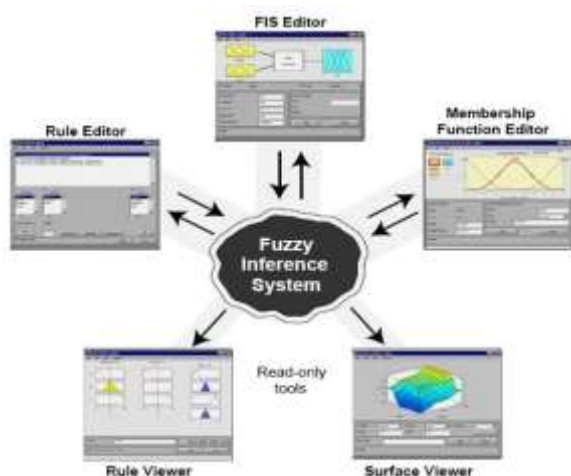
Fig.1 Graphical user interface tools in the fuzzy logic toolbox
