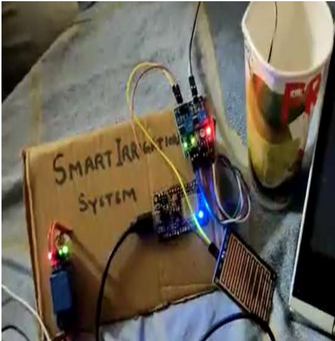
Fig 11. A fully functioning prototype of the system made to check the viability and feasibility of the model. In frame we have the rainfall sensor and Soil moisture Sensor connected with the microcontroller and functioning according to the given commands.
