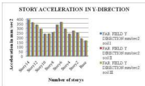
Fig 41: Shows the Story acceleration for G+12 story with different soil condition for far field earthquake.
