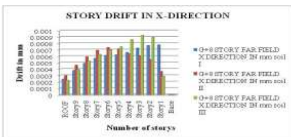
Fig 24: Shows the Story drifts for G+8 structure with different soil condition for far field earthquake.
