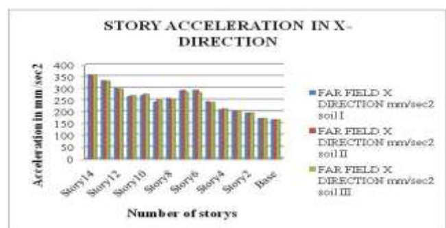
Fig 38: Shows the Story acceleration for G+12 story with different soil condition for far field earthquake.
