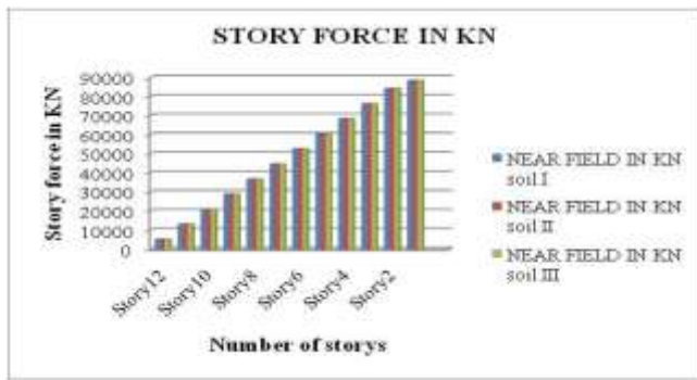
Fig 43: Shows the Story forces for G+10 story with different soil condition for near field earthquake.
