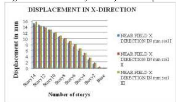
Fig 8: Shows the Story displacement for G+12 story with different soil condition for near field earthquake
