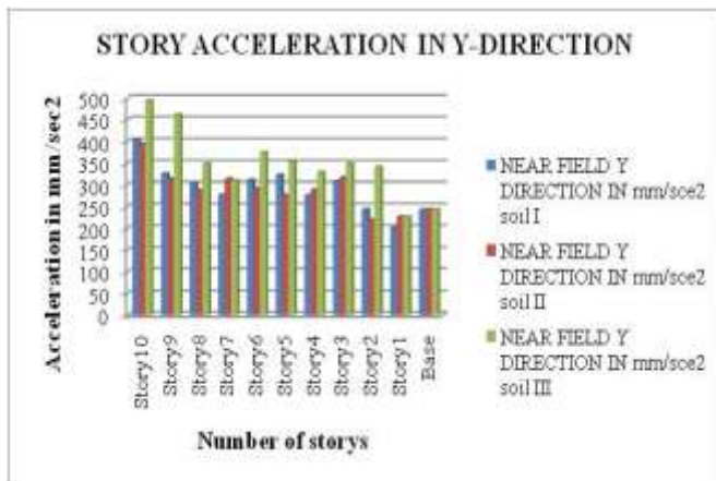
Fig 33: Shows the Story acceleration for G+8 structure with different soil condition for near field earthquake.
