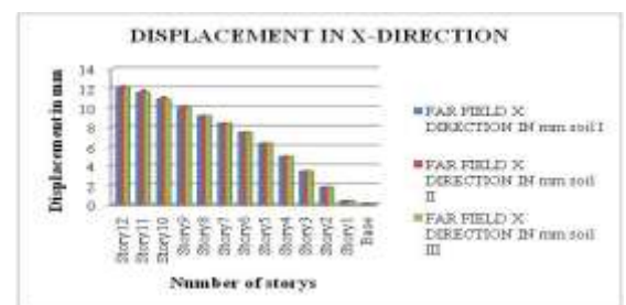
Fig 13: Shows the Story displacement for G+10 story with different soil condition for far field earthquake.
