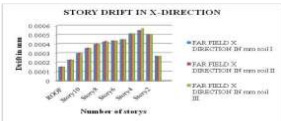
Fig 25: Shows the Story drifts for G+10 story with different soil condition for far field earthquake.
