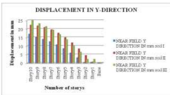
Fig 9: Shows the Story displacement for G+8 story with different soil condition for near field earthquake.
