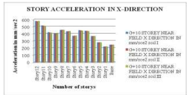
Fig 31: Shows the Story acceleration for G+10 story with different soil condition for near field earthquake.
