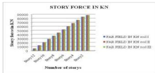
Fig 46: Shows the Story forces for G+10 story with different soil condition for far field earthquake.
