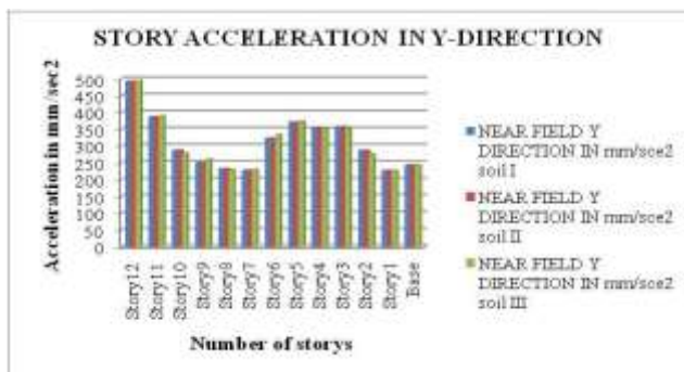
Fig 34: Shows the Story acceleration for G+10 story with different soil condition for near field earthquake.
