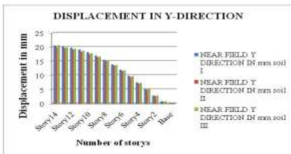
Fig 11: Shows the Story displacement for G+10 story with different soil condition for near field earthquake.
