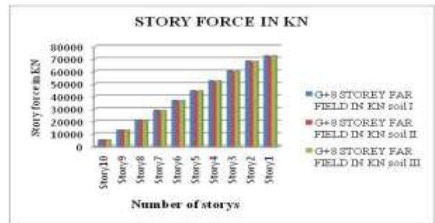
Fig 45: Shows the Story forces for G+8 story with different soil condition for far field earthquake.
