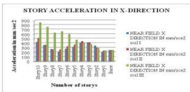
Fig 30: Shows the Story acceleration for G+8 story with different soil condition for near field earthquake.
