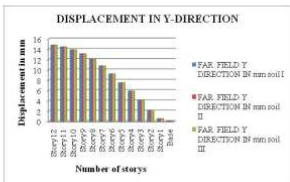
Fig 16: The Story displacement for G+10 story with different soil condition for far field earthquake.
