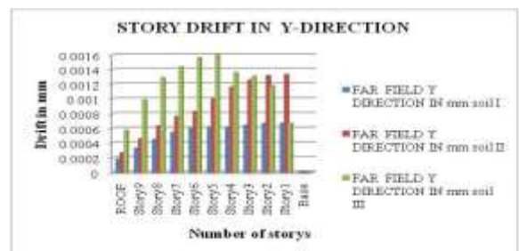
Fig 27: Shows the Story drifts for G+8 story with different soil condition for far field earthquake.
