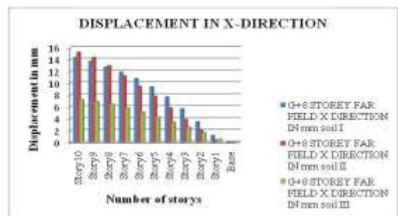
Figure 12: Shows the Story displacement for G+8 structure with different soil condition for far field earthquake.
