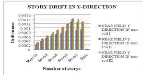
Fig 21: Shows the Story drifts for G+8 structure with different soil condition for near field earthquake.
