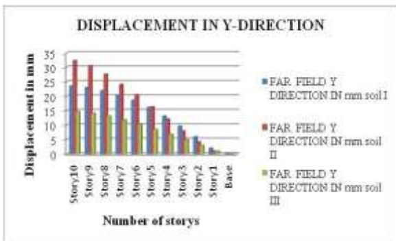
Fig 15: Shows the Story displacement for G+8 story with different soil condition for far field earthquake.
