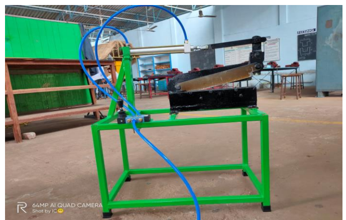
Chart -1: Pneumatic sheet metal shearing machine
