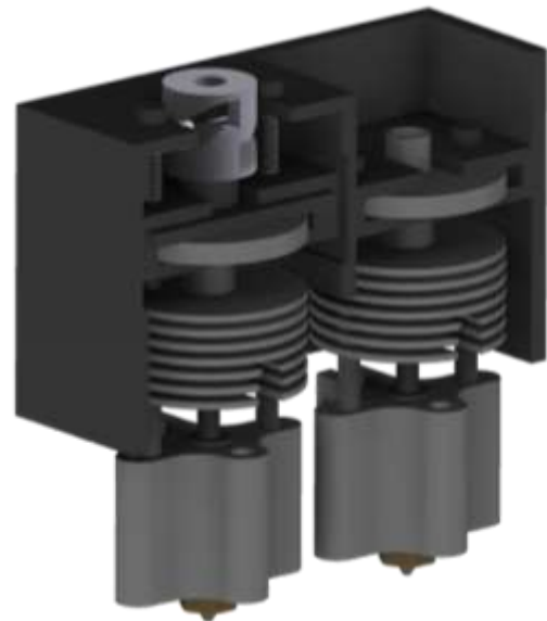
Fig. 2. 3D model of Cam operated movable hot end
