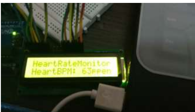
Fig 10: Result displayed on 2x16 LCD
