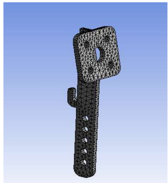
Figure-5 Meshing of Brake pedal
